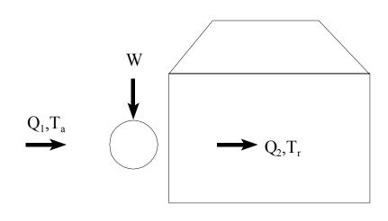
$Q_{2} = Q_{1} + W \qquad Q_{2}/T_{r} = Q_{1}/T_{a}$   $COP = Q_{2}/W = T_{r}/dT \qquad \text{where } dT = T_{r} - T_{a}$  COP is the coefficient of performanceIt is the inverse of the Carnot efficiency
