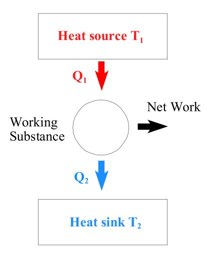
All heat,  $Q_1$ , enters at  $T_1$  and all waste heat,  $Q_2$ , leaves at  $T_2$ .
